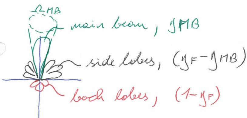
main beam efficiency:  $\gamma_{MB} = \frac{\mathcal{R}_{MB}}{\mathcal{R}_A}$
