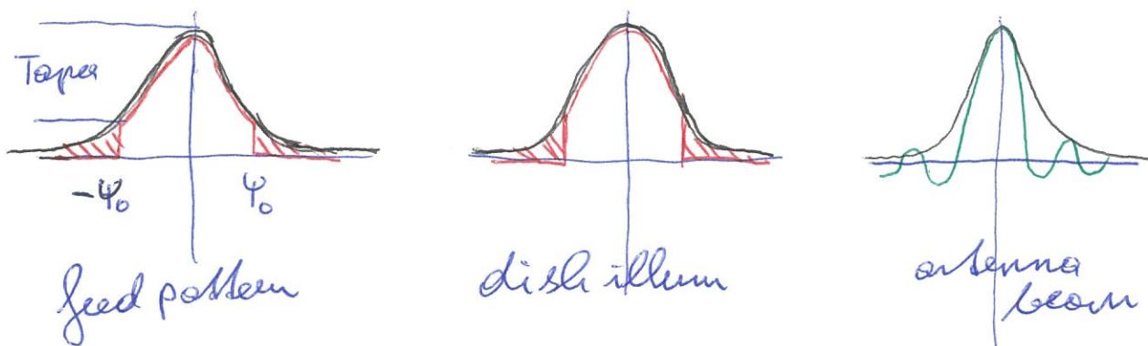
$T = \infty \rightarrow$  gaussian feed pattern  $\rightarrow$  gaussian dish illum.
